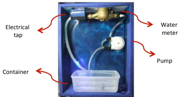
Figure 3 Simulating a water consumer installation: water meter, pump, container and electrical tap
